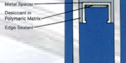
Intercept Insulating Glass Warm Edge Construction
