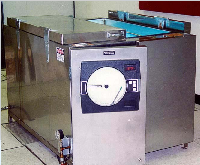
High heat and humidity chamber above tortures the sealed IGU 24 hours every day for six months to simulate over 20 years in the “real world”
